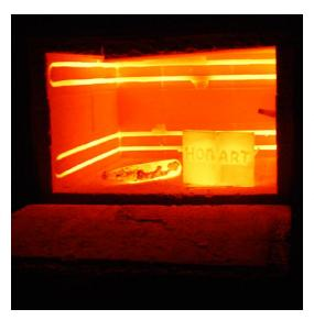
Annealing (...) is a process that produces conditions by heating to above the re-crystallisation temperature and maintaining a suitable temperature, and then cooling. - Wikipedia
